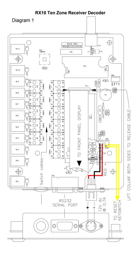
Note! When re-fitting the front panel ribbon cable, ensure that the connector collar is raised and check that the cable is square to the connector. Ensure that the cable runs straight in the direction shown. Gently insert the cable tail as far as it will go, then push down equally on both sides of the connector collar.
