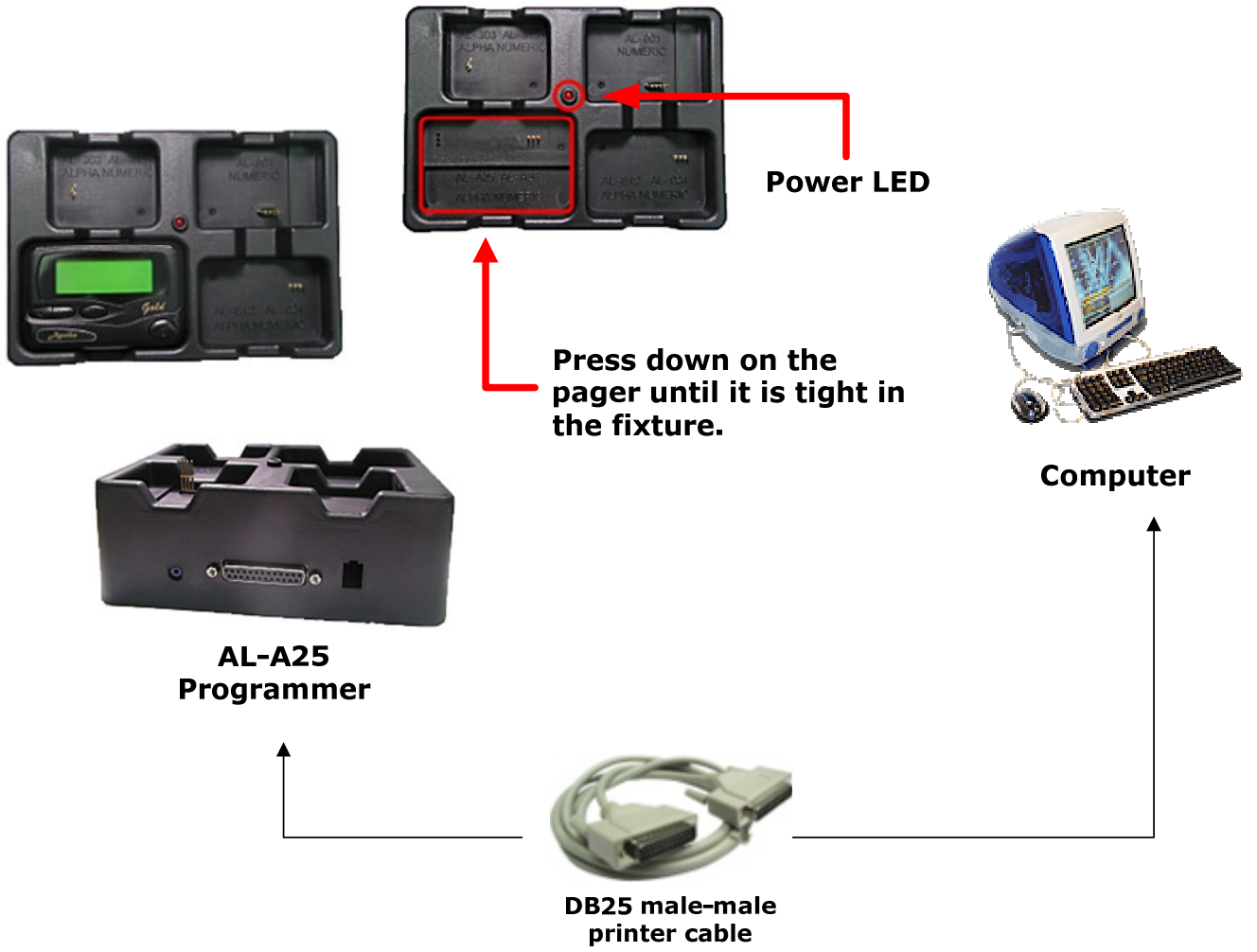
Figure 1 Programmer Hardware Connections
